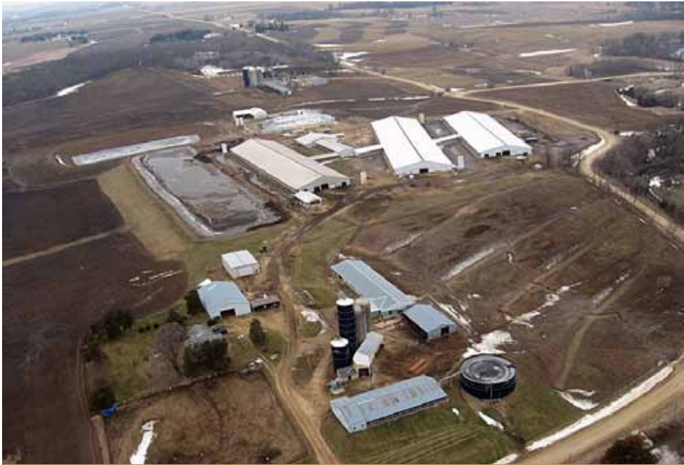
Aerial view of Rancho Cantera dairy in Stephenson County, Illinois. The large round tank at the bottom of the photo holds liquid manure until it can be spread onto nearby fields. (See below.)
